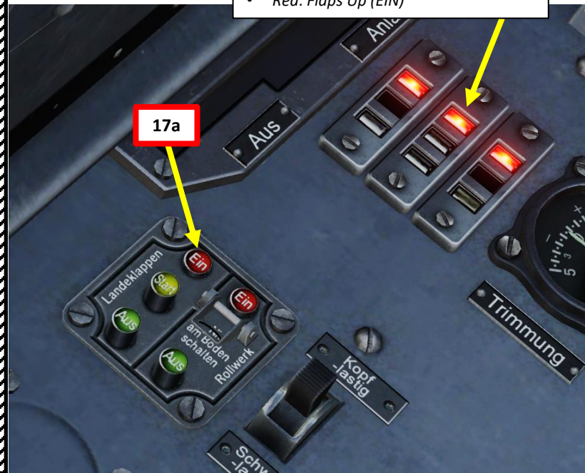
Flaps Position Indicator Light • Green: Flaps Down (AUS) • Amber: Flaps Takeoff/START Position • Red: Flaps Up (EIN)
