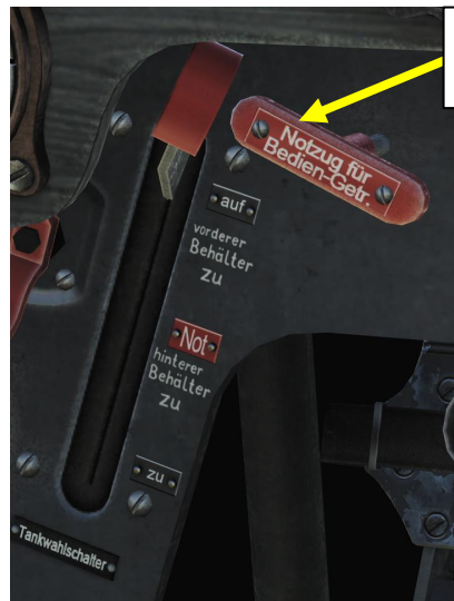
MBG (Motorbediengerät, or Engine Control Unit) Emergency Mode Handle
