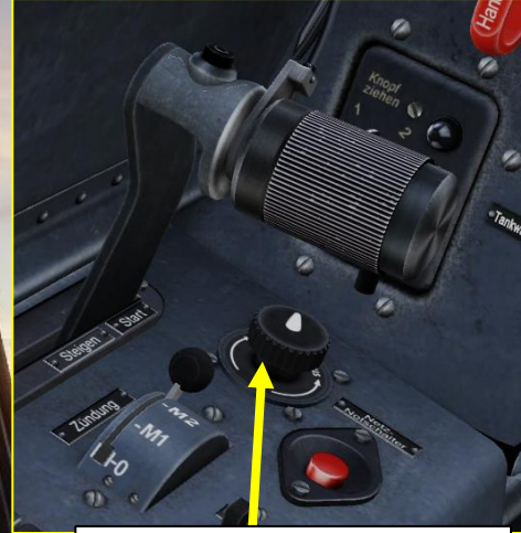
Instruments Lights Brightness Control Knob
