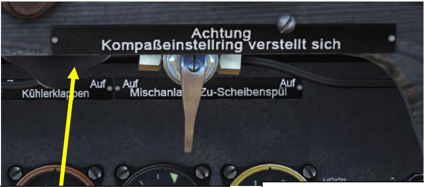
Manual Radiator Flap Control • Clockwise / Auf = Open • Counter-clockwise / Zu = Closed
