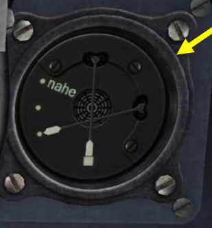
Supercharger Pressure Gauge (ATA) • Similar to Boost or Manifold Pressure
