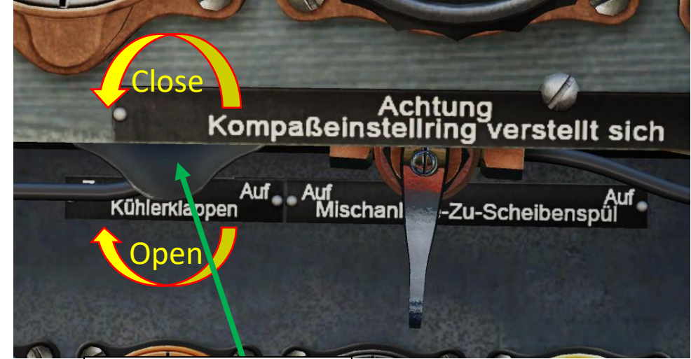
Manual Radiator Flap Control
